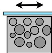
Non-penetrating product sits on top of concrete to form an external film on surface.
